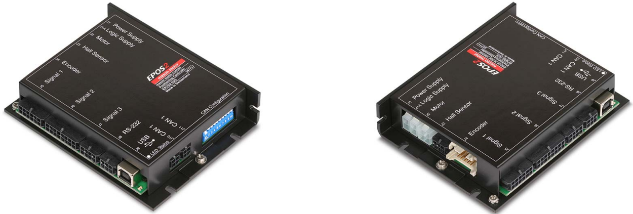
Figure 4-4 Interfaces – Designations and Location
