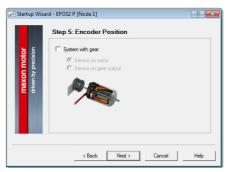
Figure 3-22 Startup Wizard Dialog for DC Motors: Encoder Position
